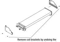
Remove coil brackets by undoing the 4x M5 hex bolts, rotate coil to opposite handing and re-attach brackets
